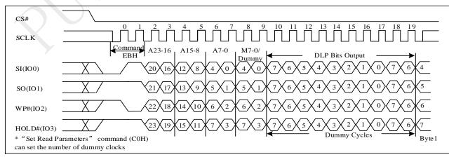
Figure 10-30f 4IO Read with DLP bits output Sequence (QPI)
