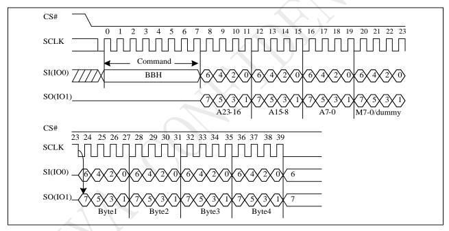
Figure 10-20 2IO Read Sequence (SPI, M5-4 ≠ (1,0))
