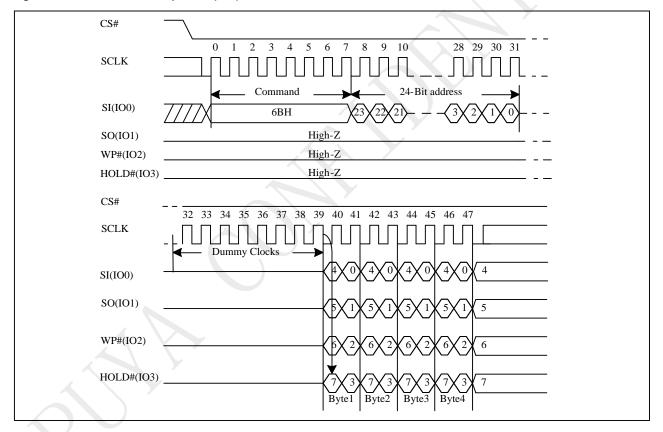
Figure 10-23 Quad Read Sequence (SPI)
