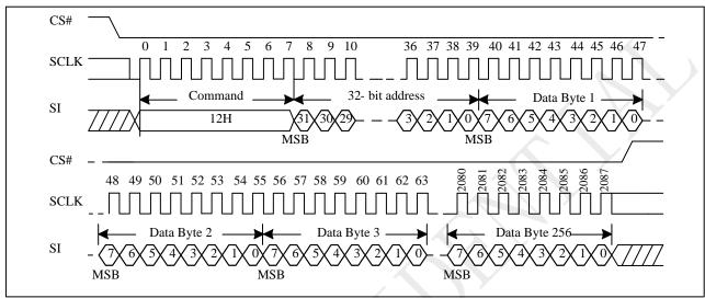
Figure 10-41 Page Program with 4-Byte Address Sequence (SPI)
