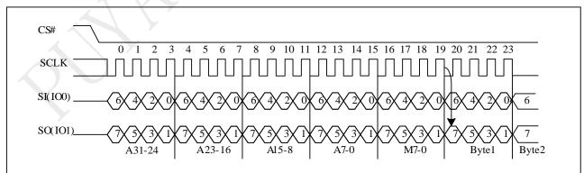
Note:2IO Continue Read with 4-Byte Address, if M5-4 = 1, 0. If not using Continue Read recommend to set M5-4  $\neq$  1, 0.
