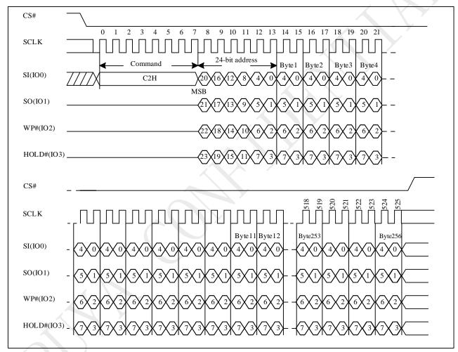
Figure 10-44 Quad Page Program (QPP) Sequence (SPI)
