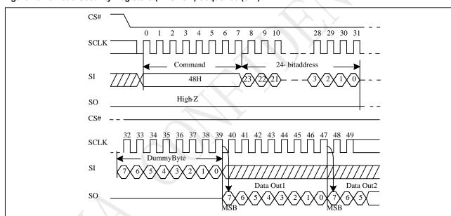
Figure 10-48 Read Security Registers (RDSCUR) Sequence (SPI)
