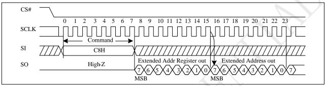
Figure 10-9a Read Extended Address Register Sequence (QPI)
