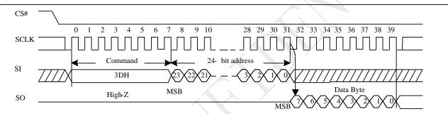
Figure 10-61 Read Block Lock Status (SPI)
