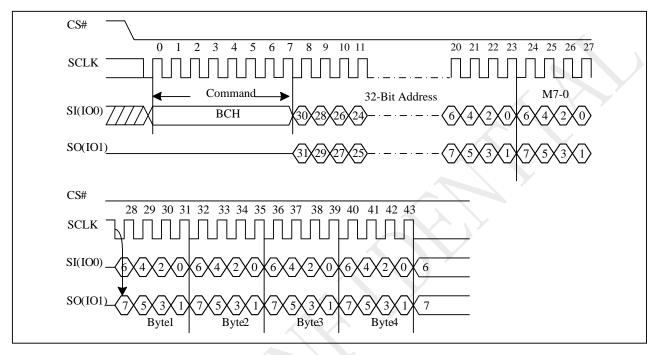
Figure 10-22 2IO Read with 4-Byte Address Sequence (SPI, M5-4 ≠ (1,0))
