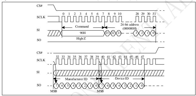
Figure 10-51 Read Electronic Manufacturer & Device ID (REMS) Sequence (SPI)
