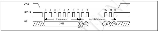
Note: 32-bit address is required when the device is operation in 4-byte address mode.
