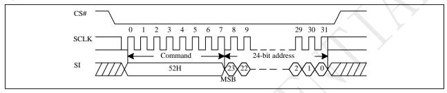
Note:32-bit address is required when the device is operation in 4-Byte Address Mode.
