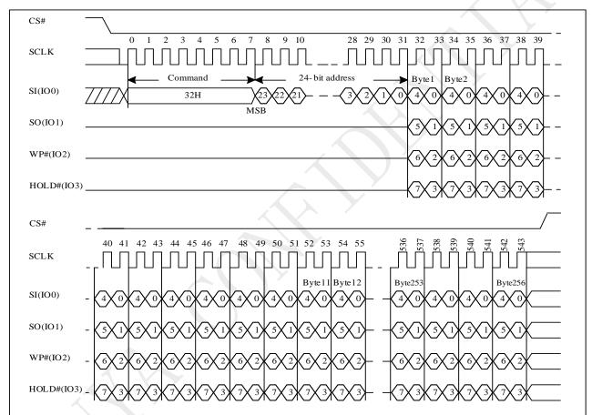
Figure 10-42 Quad Page Program (QPP) Sequence (SPI)
