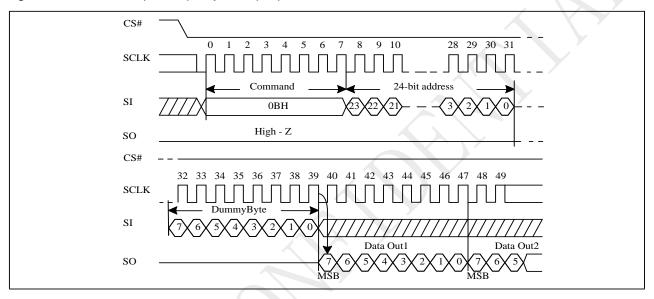
Figure 10-15 Fast Read (FREAD) Sequence (SPI)
