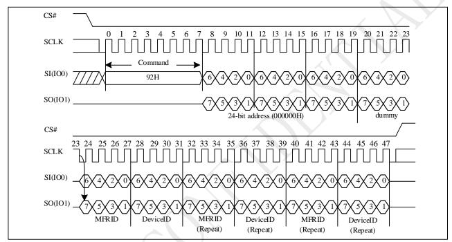
Figure 10-52 DUAL I/O Read Electronic Manufacturer & Device ID (DREMS) Sequence (SPI)
