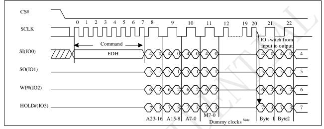
Figure 10-27 DTR 4IO Read Mode Sequence (SPI, M5-4 ≠ (1,0))
